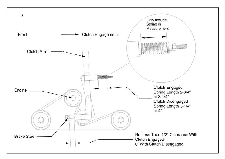
Figure 10: Belt Pattern, Spring Adjustment, and Brake Adjustment
